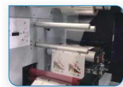
Lamination & Lamination liner removal
